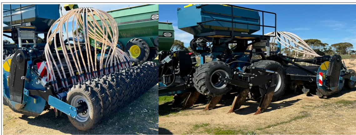
The spader used for ameliorating the soil. The front view shows the clay delving tynes that lift the clay to the surface, followed by the mixing action of the spader and then the seeder to place the seed and fertiliser, with the press wheels to firm the seedbed and assist with germination.
