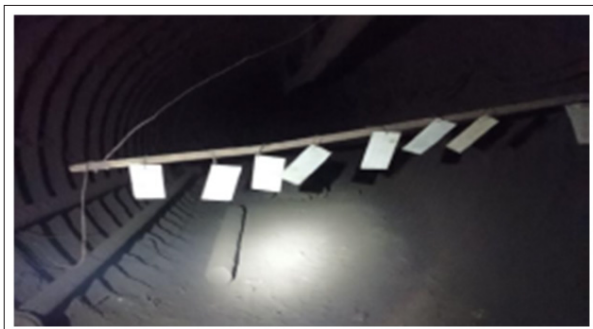
Figure 2: Measurement of airborne dust with dust tables
